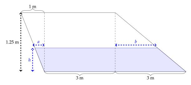
• The triangle on the left has height *h* metres. Let its base be *a* metres. It forms a similar triangle with the triangle whose height is 1.25 metres and width is 1 metre, so:
