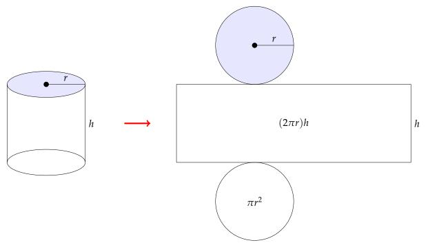
So, the surface area is  $2\pi r^2 + 2\pi rh$ . Since the area is given as *A*, we can solve for *h*:
