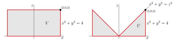
(a) In cylindrical coordinates,  $x^2 + y^2 \le 4$  becomes  $r \le 2$  and  $x^2 + y^2 \ge z^2$  is  $r \ge |z|$ , and the density is  $\sqrt{x^2 + y^2} = r$ . So
