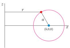
$(r-b)^2+z^2=a^2$ . (Recall that the cylindrical coordinate r of a point is its distance from the z-axis.) On this torus,
