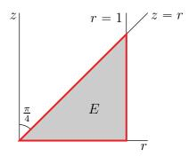
Recall that the spherical coordinate  $\varphi$  is the angle between the z-axis and the radius vector. So, in spherical coordinates z=r (which makes an angle  $\frac{\pi}{4}$  with the z axis) becomes  $\varphi=\frac{\pi}{4}$ , and the plane z=0, i.e. the xy-plane, becomes  $\varphi=\frac{\pi}{2}$ , and r=1 becomes  $\rho\sin\varphi=1$ . So
