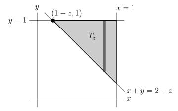
In setting up the domain of integration, we'll decompose, for each  $0 \le z \le 1$ ,  $T_z$  into vertical strips as in the figure above. On  $T_z$
